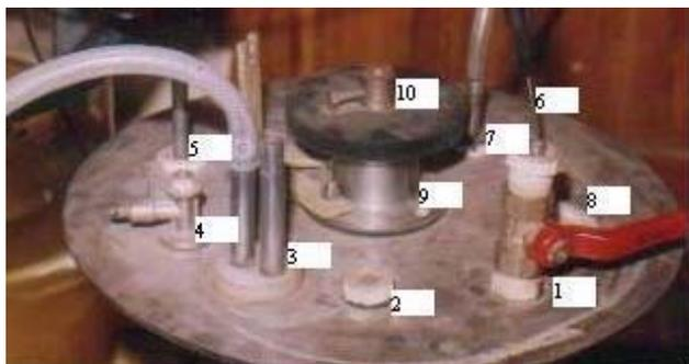
**Figure 2.** Stainless top plate. 1. Feed port; 2. Acid/alkali port; 3. Cooling water port; 4. Gas exhaust port; 5. Sampling port; 6. Temperature probe; 7. Aeration port; 8. pH probe port; 9. Support for agitation shaft; 10. Gear coupled to the shaft.
